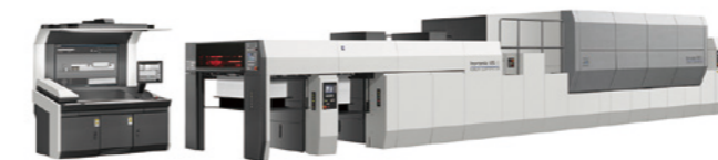
Impremia NS40 with Nanographic Printing® technology that enables high-resolution printing
